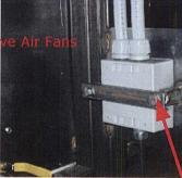
The back of the switch box, this bar pushes the box to the switch plate. The right and left corner post are the first post you need to locate
